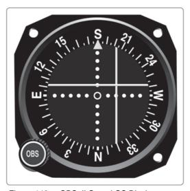
Figure 142. – OBS, ILS, and GS Displacement.
