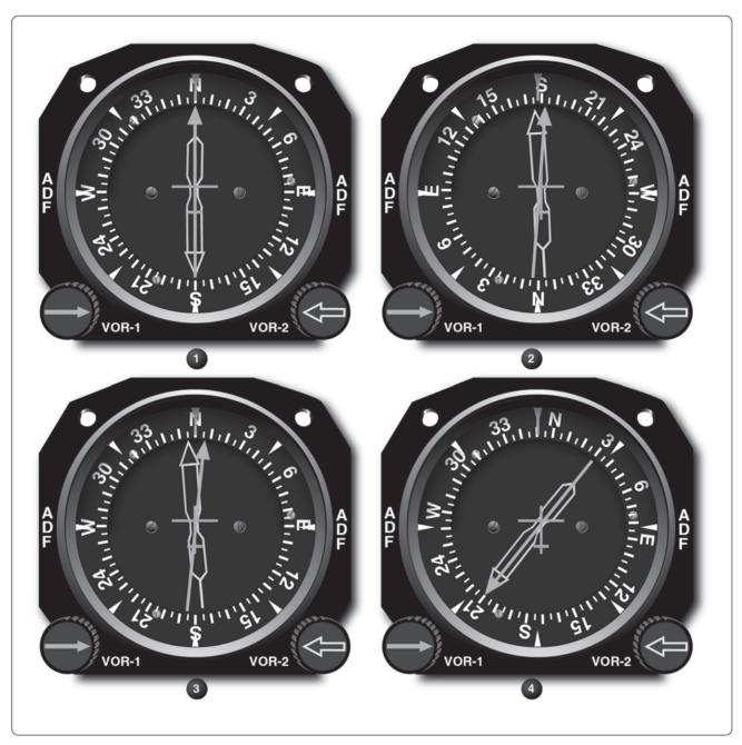
Figure 82. – Dual VOR System, Accuracy Check.
